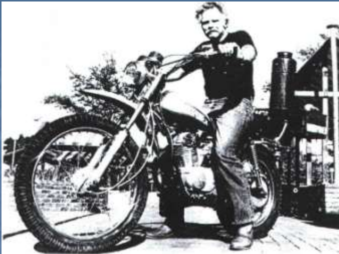
Gainesville, Florida, 1981. The tiny generator that powers this wood-burning motorcycle was constructed at the University of Florida out of a fire-extinguisher casing. The vehicle gets 70 km per kg of wood (20 miles per lb). (Sun Photo by Barbara Hansen)
