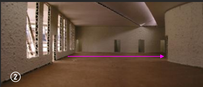
Daylighting model to test effectiveness of clerestories
