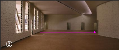
Daylighting model to test effectiveness of clerestories
